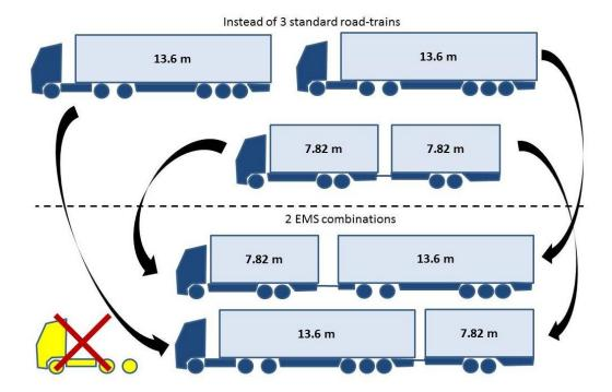
This means an overall reduction of the number of trucks on the road by as much as 33%. The EC has introduced the principle of subsidiary when it comes to the use of the modular concept. In accordance to Article 4 Number 4 "Member States may allow" vehicles or vehicle combinations with deviating dimensions.
