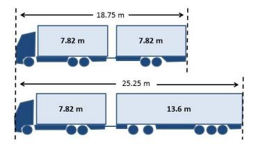
The main advantage of EMS is that in cases where the amount of freight to be transported would require two or more standard lorries to be used, the use of an EMS vehicle would allow to reduce the number of trucks by 1/3.
