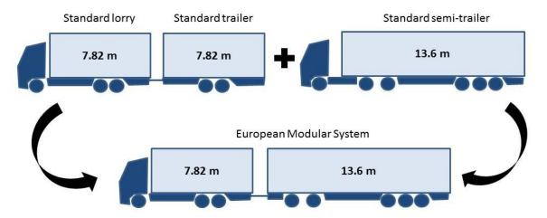
The European Modular System, therefore, does neither mean that the lorries are longer ("megatrucks"), nor that the trailers are longer. EMS uses **standard modules only**.
